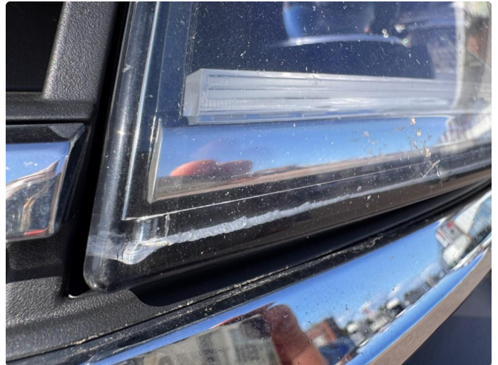
2.1 Krakelering i plast
