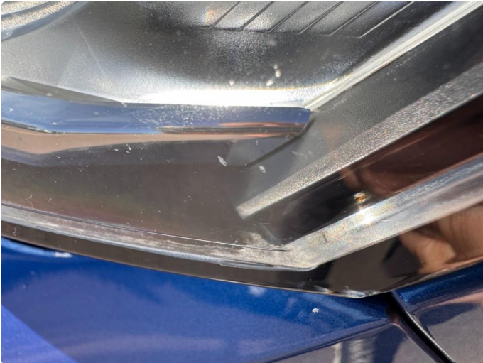
2.1 Krakelering i plast
