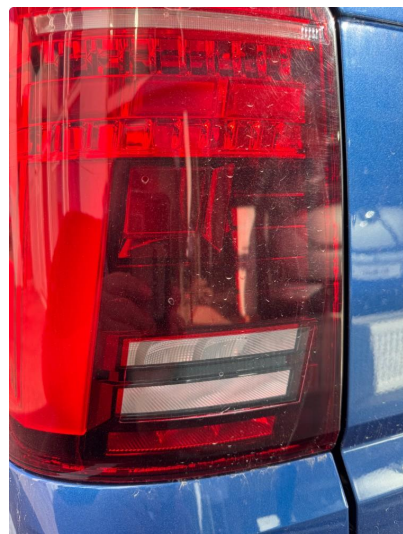
2.2 Krakelering i plast
