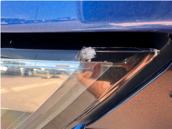
2.1 Krakelering i plast
