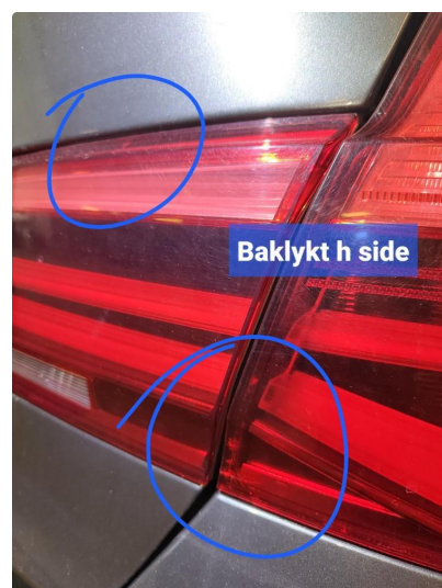
2.1 Krakelering i plast
