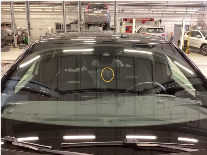
1.2 Liten steinsprut utover synsfelt, trenger ikke rep.
