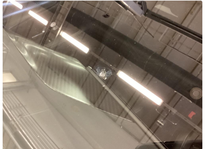
1.2 Liten steinsprut utover synsfelt, trenger ikke rep.
