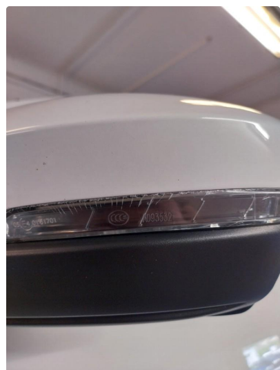
2.1 Krakelering i plast
