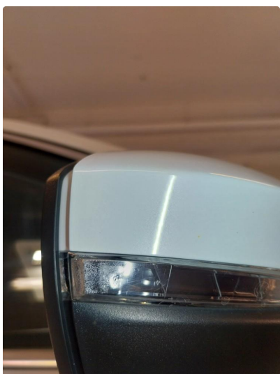
2.1 Krakelering i plast
