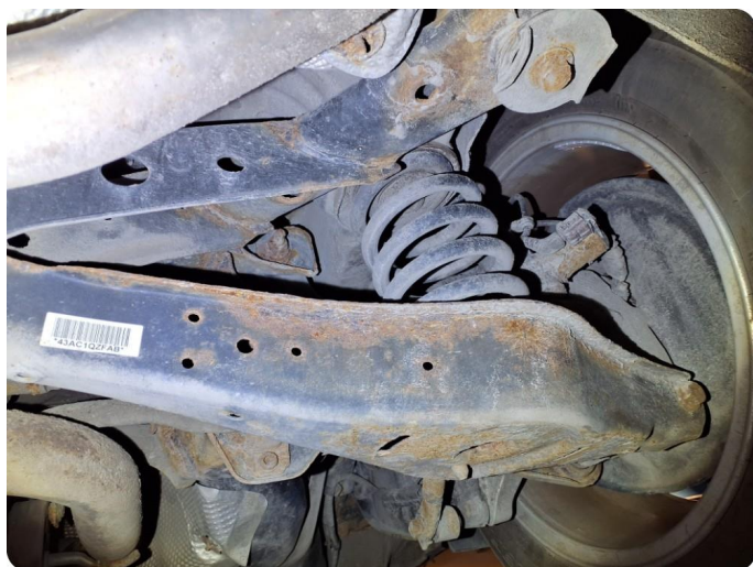
2.2 Rust (Til info)
