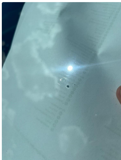
1.1 Steinsprut i synsfelt
