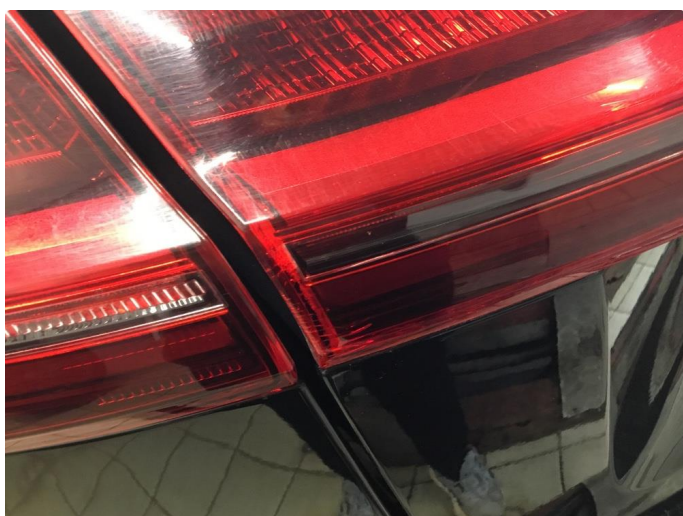
2.1 Krakelering i plast
