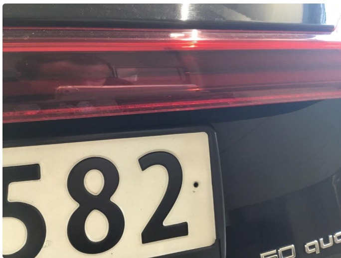
2.1 Krakelering i plast
