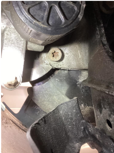
2.1 Mer enn 25% rust
