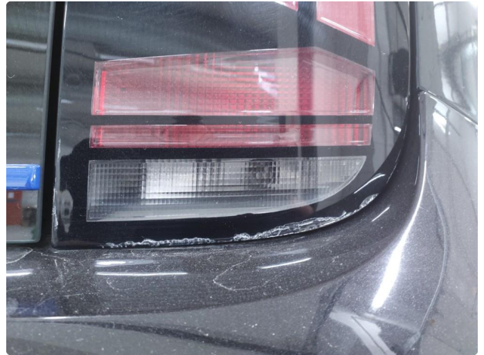
2.1 Krakelering i plast
