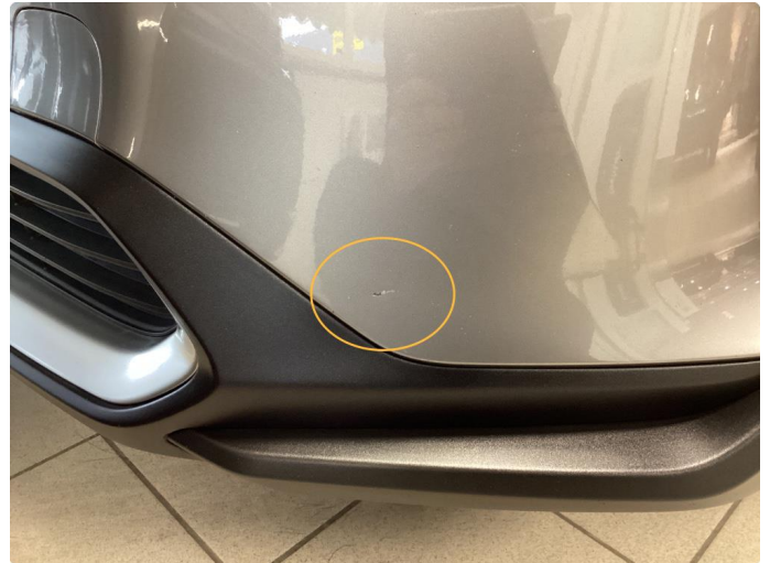
1.2 Steinsprut h foran
