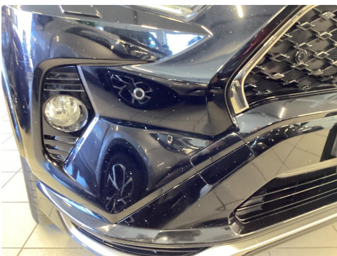
1.5 Steinsprut fanger foran
