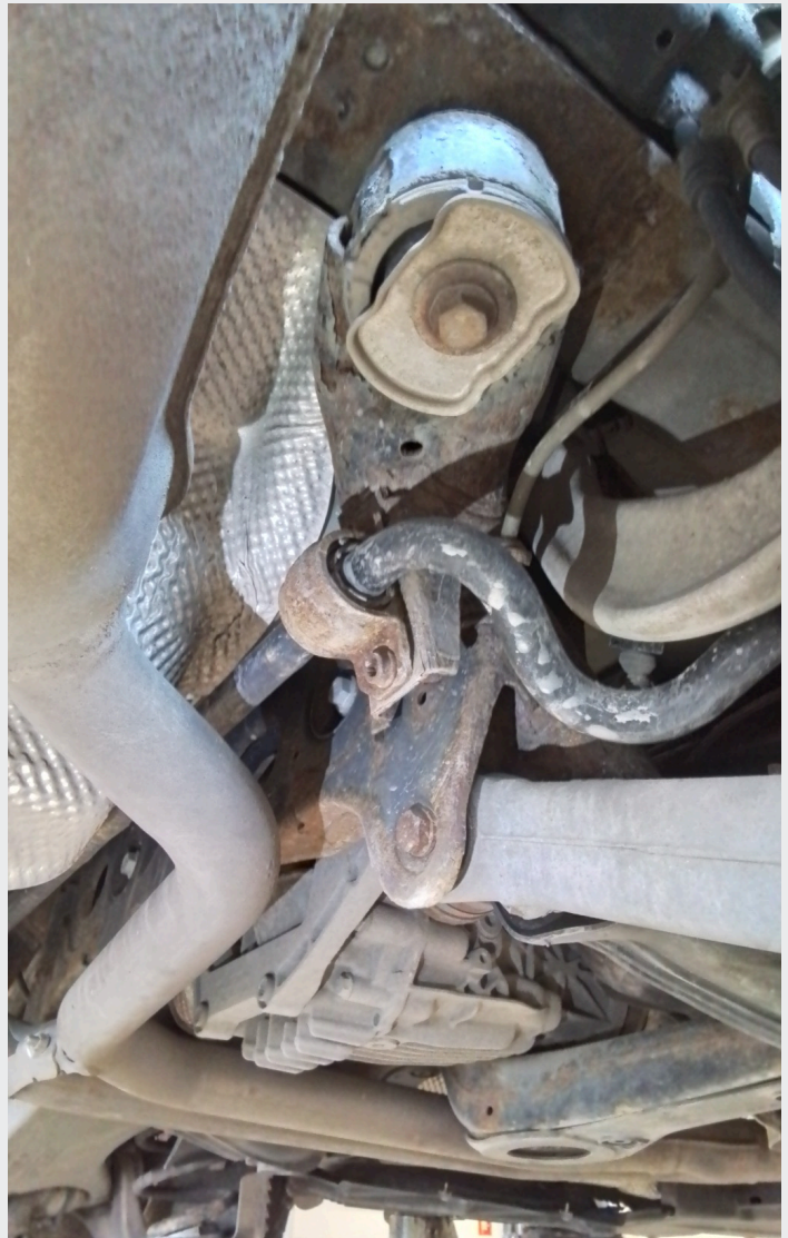
2.2 Noe rust travers bak
