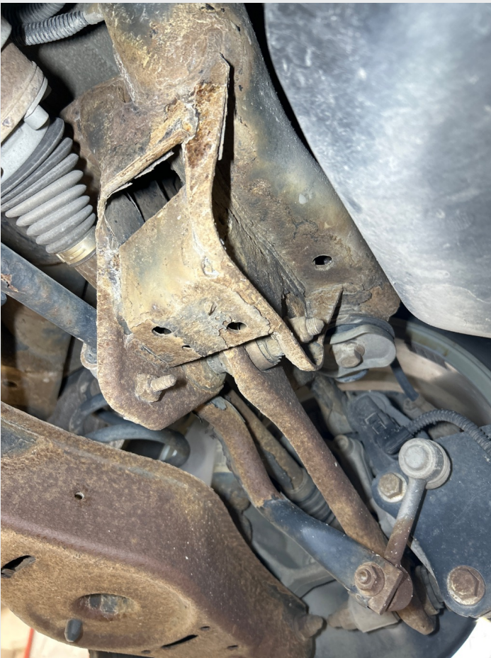
2.14 Rust finnes, travers bak
