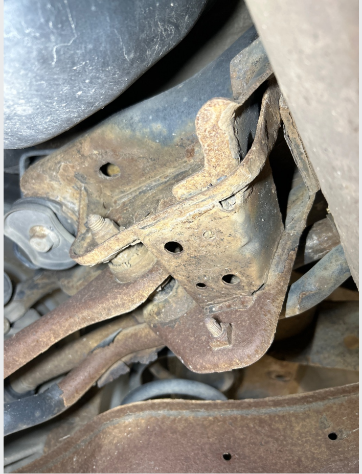
2.14 Rust finnes, travers bak
