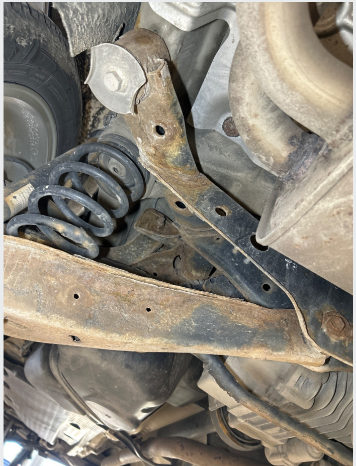
2.14 Rust finnes, travers bak
