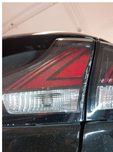
2.1 Krakelering i plast
