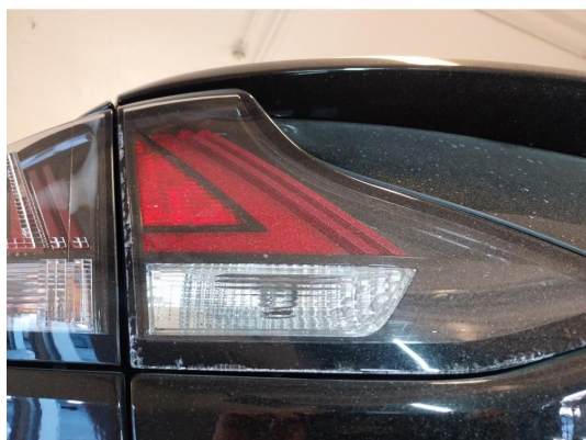
2.1 Krakelering i plast
