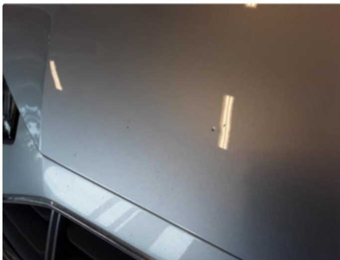
1.1 Noe steinsprut i front.
