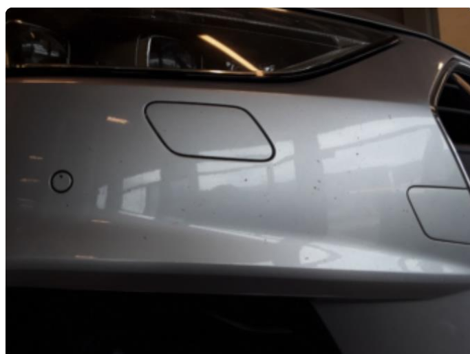
1.1 Noe steinsprut i front.
