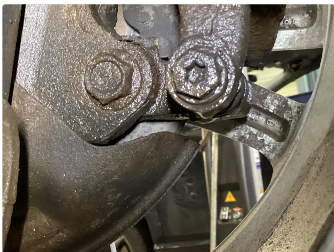
2.2 Mer enn 25% rust
