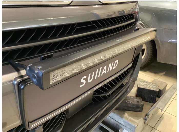
2.1 Fukt i lysbjelke
