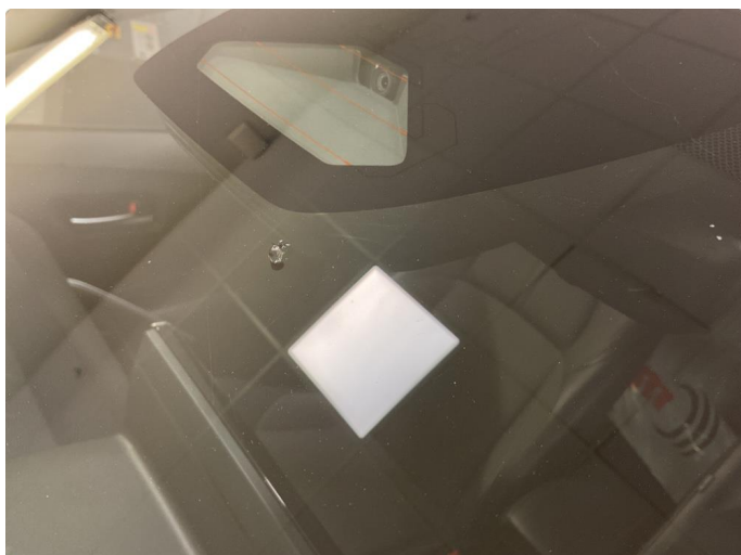
1.1 Steinsprut utenfor synsfelt
