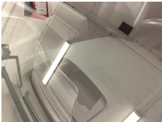
1.3 Steinsprut utenfor synsfelt
