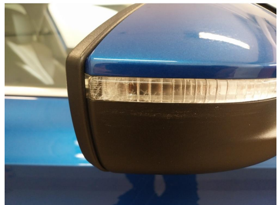
2.1 Krakelering i plast
