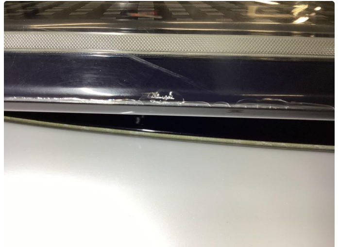
2.1 Krakelering i plast
