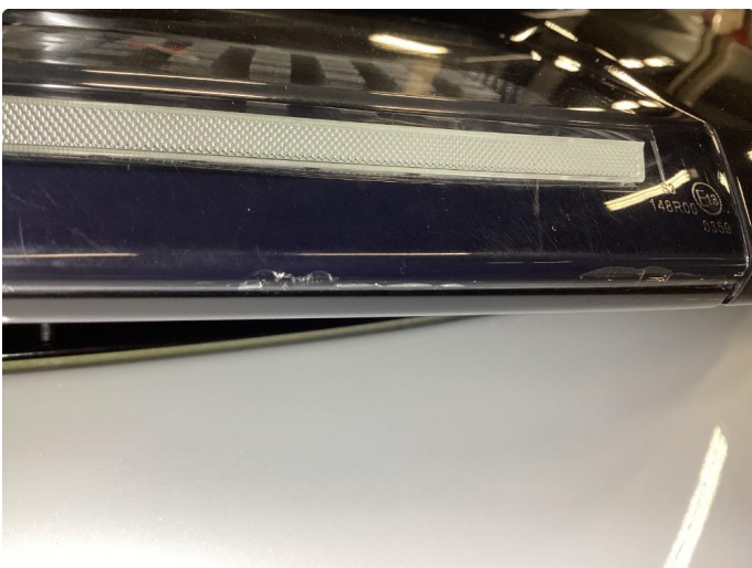
2.1 Krakelering i plast
