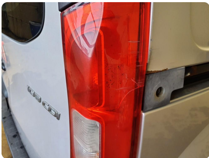
4.4 Defekt / sprukket glass
