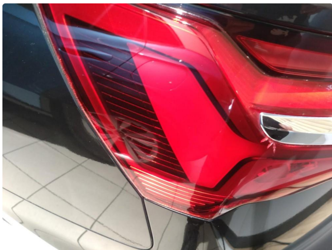
2.1 Krakelering i plast
