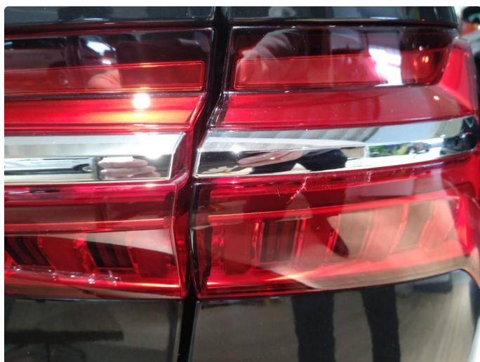
2.1 Krakelering i plast
