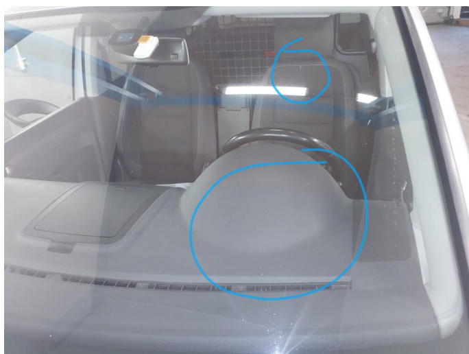
1.12 Steinsprut i synsfelt
