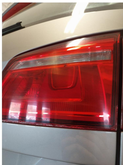
2.1 Krakelering i plast
