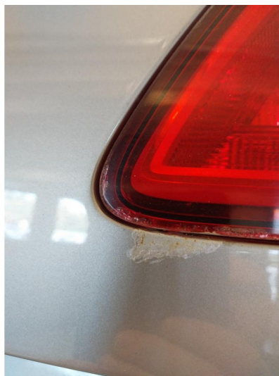
2.1 Krakelering i plast
