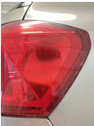
2.1 Krakelering i plast
