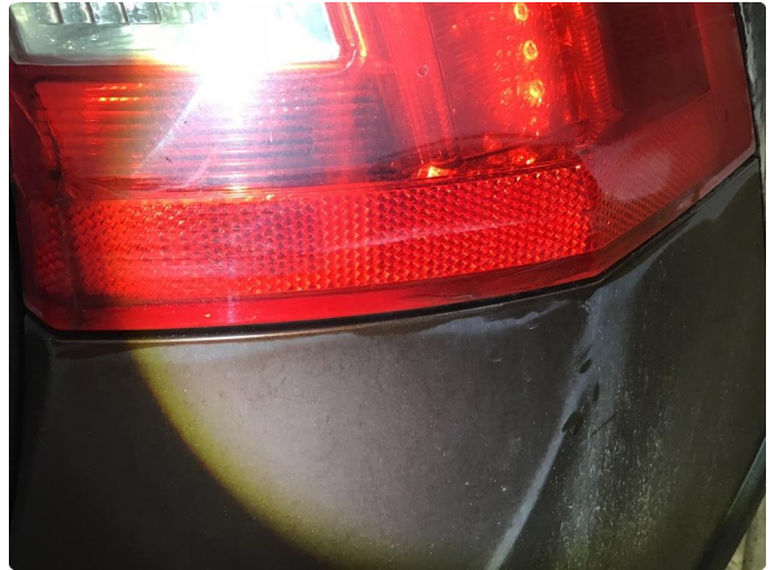
2.1 Krakelering i plast
