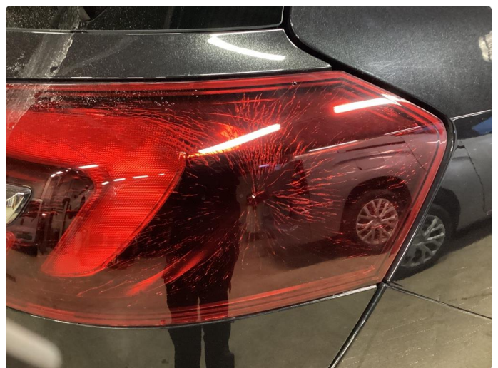
2.1 Krakelering i plast
