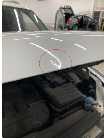
1.1 Liten bulk i panser. Steinsprut penslet m/lakk
