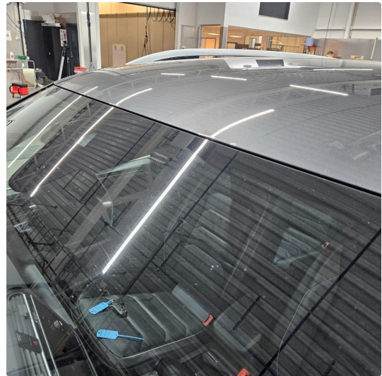
1.2 Steinsprut fremkant, blitt penslet m/lakk
