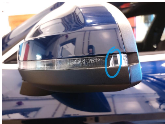
2.1 Krakelering i plast
