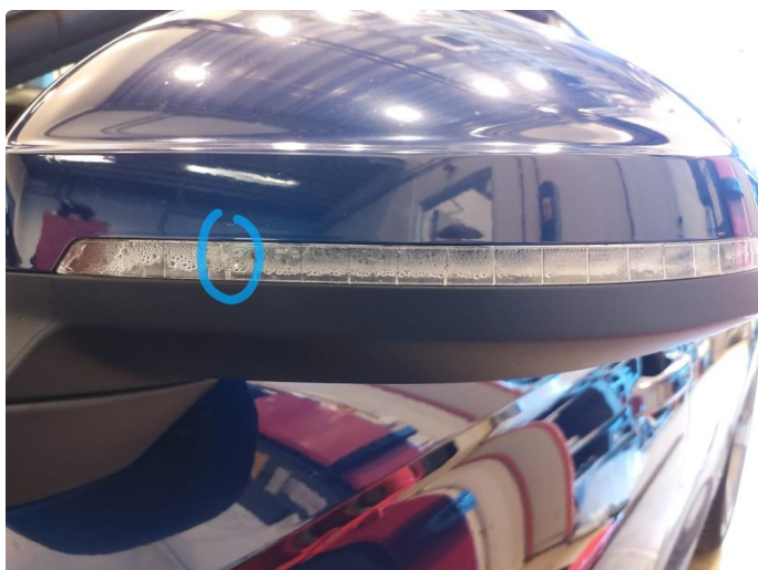
2.1 Krakelering i plast
