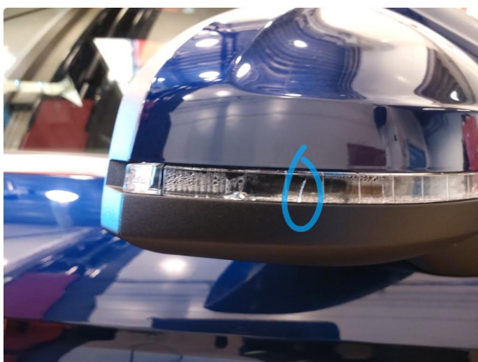
2.1 Krakelering i plast
