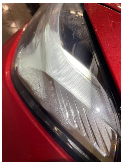
2.1 Dugg/fukt (byttes garanti)
