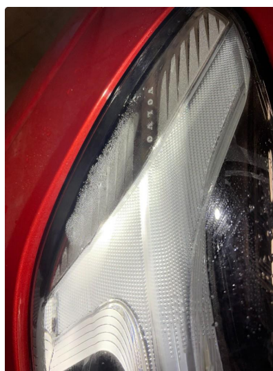
2.1 Dugg/fukt (byttes garanti)
