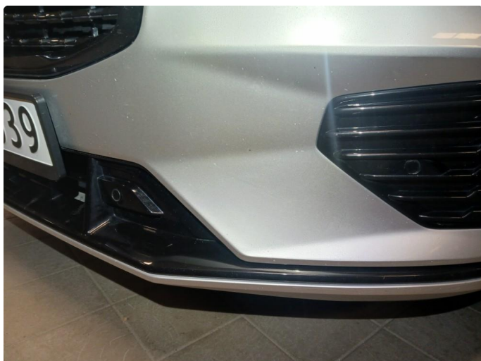
1.1 Noe stensprut i front
