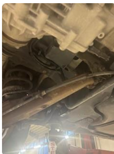
1.2 Noe overflaterust under bil
