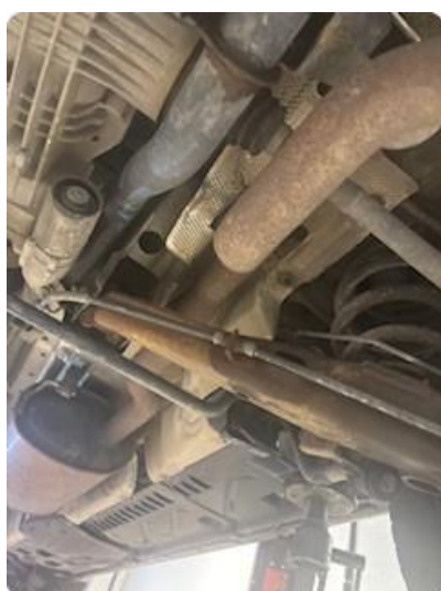
1.2 Noe overflaterust under bil
