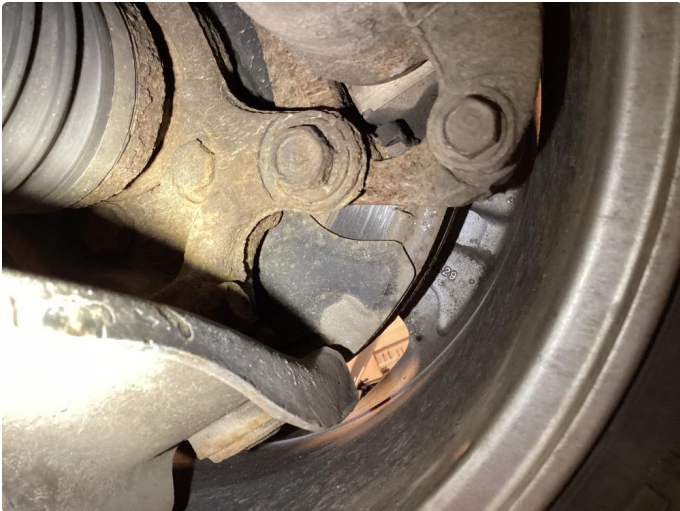
4.2 Mer enn 25% rust innside skiver foran.
