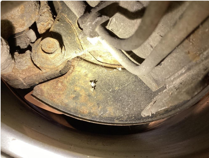
4.3 Mer enn 50%rust innside skive VSB
