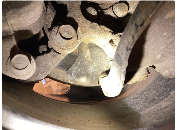
4.2 Mer enn 25% rust innside skiver foran.
