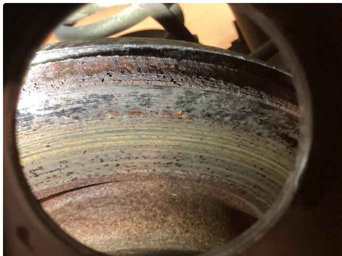
1.2 Mer enn 50% rust utside skive hsb.
