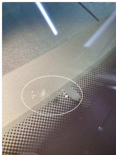
1.2 Steinsprut, nedre del, rep./limt OK (for info)
