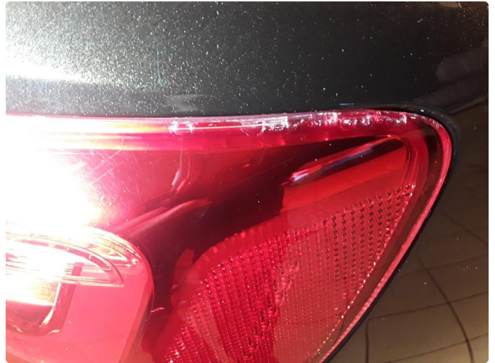
2.1 Krakelering i plast
