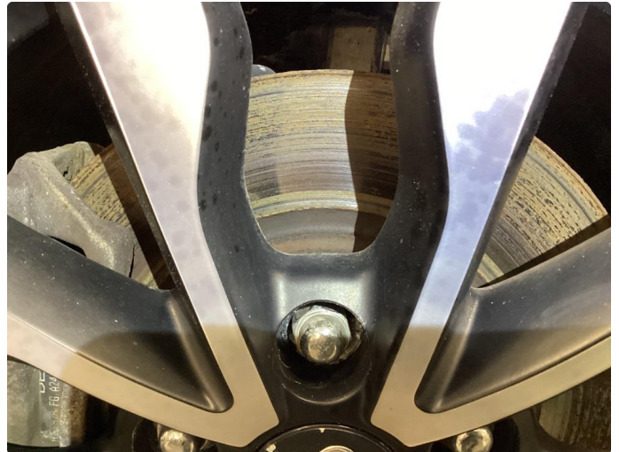
1.1 Mer enn 25% rust
