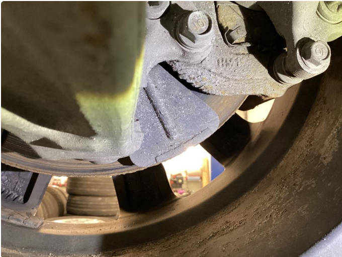
1.1 Mer enn 25% rust
