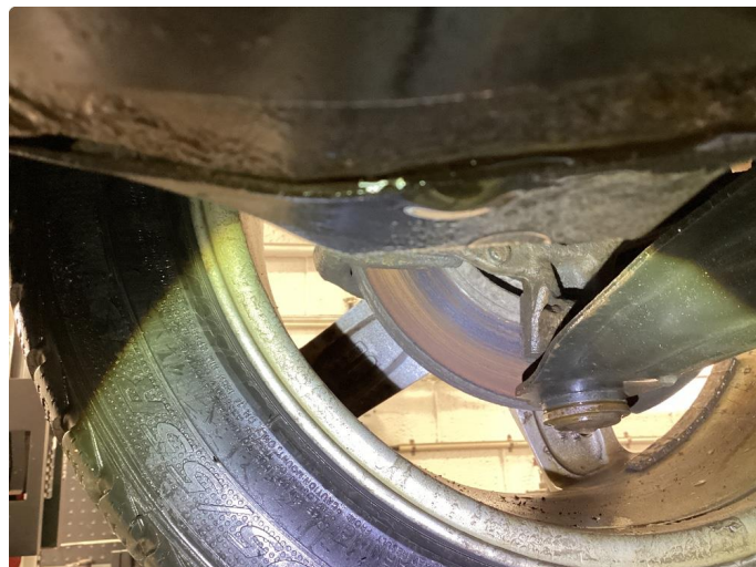
2.1 Mer enn 25% rust
