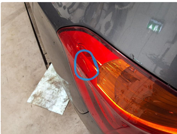
2.2 Krakelering i plast
