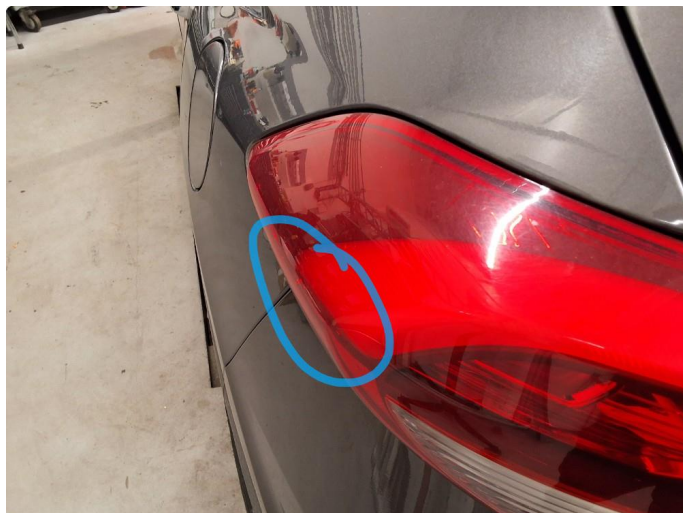
1.2 Krakelering i plast
