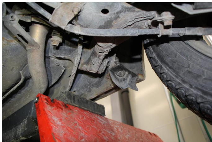
1.2 Litt rust i chassiss
