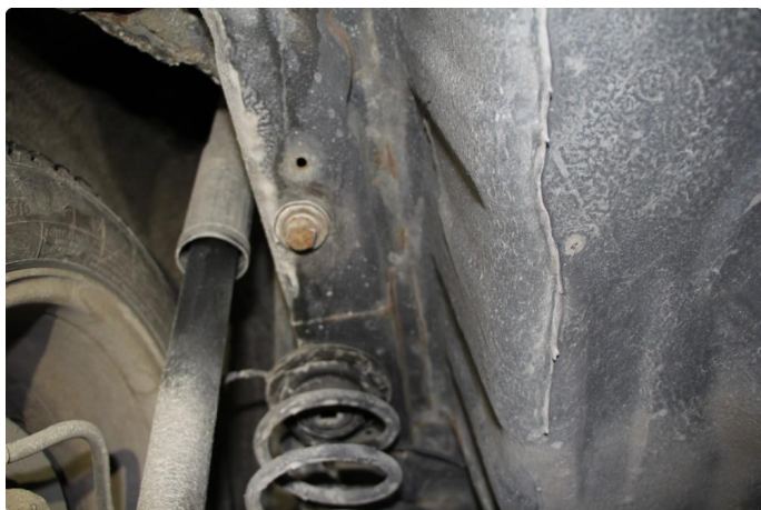
1.2 Litt rust i chassiss
