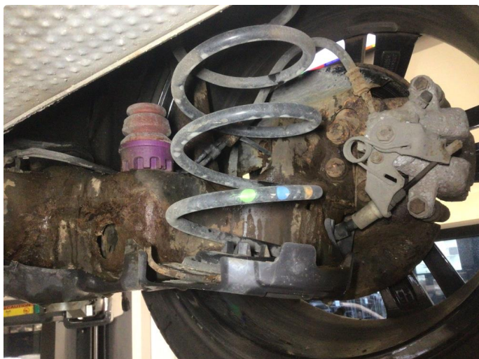
2.1 Overflaterust i bakstilling
