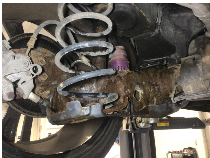
2.1 Overflaterust i bakstilling
