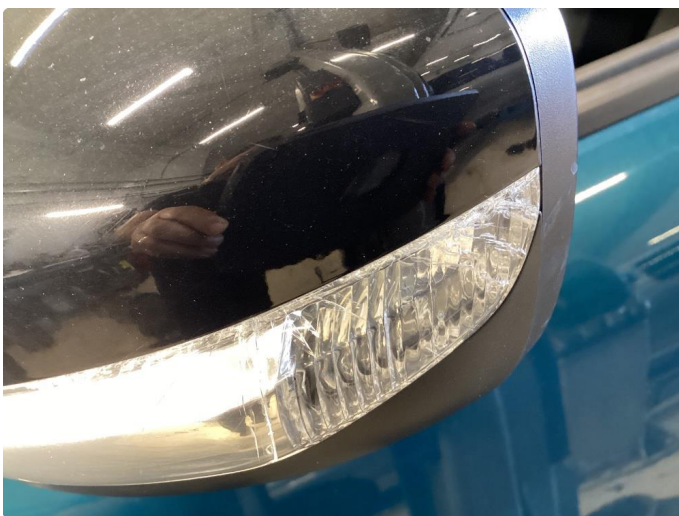
2.1 Krakelering i plast
