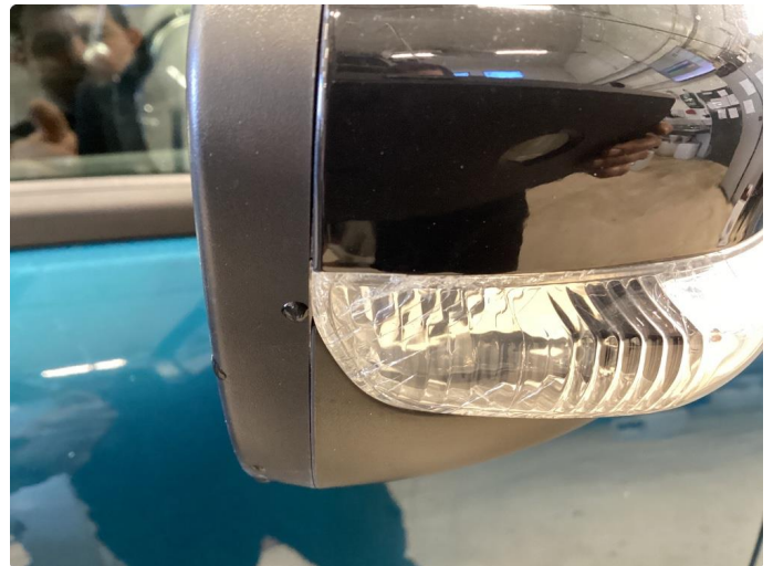
2.1 Krakelering i plast
