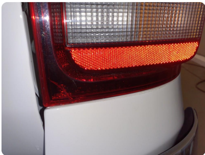
4.1 Krakelering i plast Krakelering I baklamper
