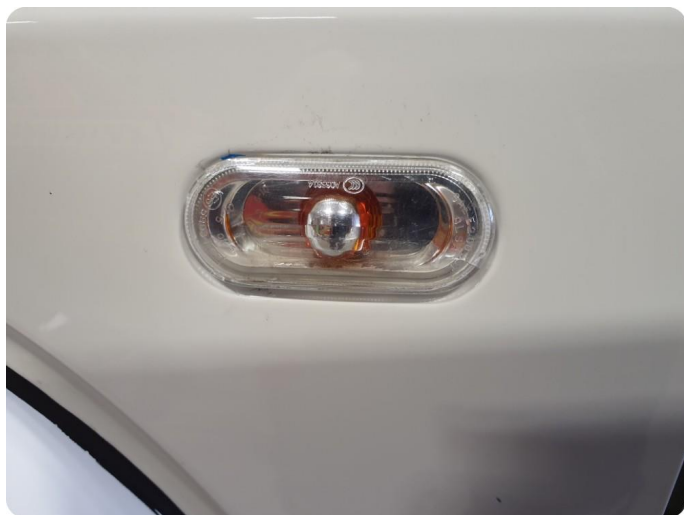
4.2 Krakelering i plast Krakelering I side blinklys
