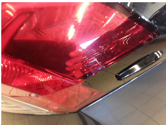
2.1 Noe krakelering i plast.
