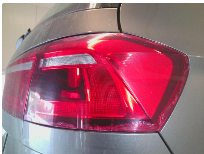
2.1 Krakelering i plast
