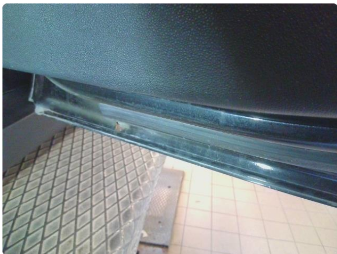
2.5 Rust i fals
