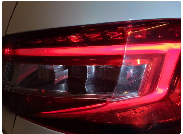
2.1 Noe krakelering i plasten
