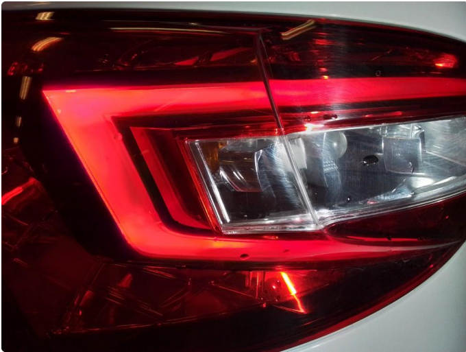
2.1 Noe krakelering i plasten
