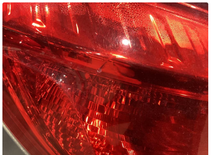
2.1 Krakelering i plast
